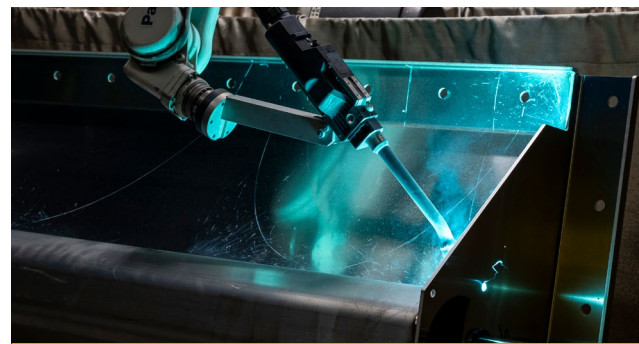
Fabrication & Robotoc Welding
